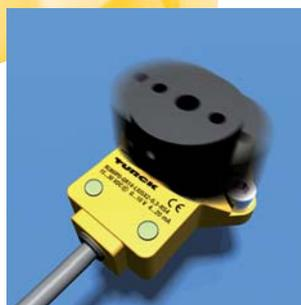
The new angle sensors provide highly precise measuring signals within  $360^\circ$  and a repeatability of  $0.09^\circ$ . Bearing tolerances are easily compensated through the contactless principle, as well as vibration caused by irregularly rotating shafts. This guarantees high linearity
