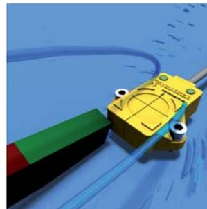
Frequency converters, large motors, ferritic metals or permanent magnets are no problem at all. The new angle sensor operating on the basis of resonance oscillation, is insensitive to interference caused by magnetic fields and features excellent EMC properties. The distance between sensor and positioning element as well as roughness in the guidance have no influence on the output signal.
