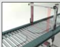
Clear plate glass profiling (Measure width of glass)
