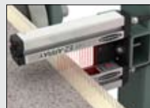
Air-to-backing and backing-to-tufting monitoring
